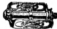
No. 46 Course and Cyclotouriste World patented design giving a choice of reach simply by reversing the pedal. The concave side gives a rational support for the foot and the reverse side being flat allows a relaxation of the leg. 3½" wide, 15oz. pair.
